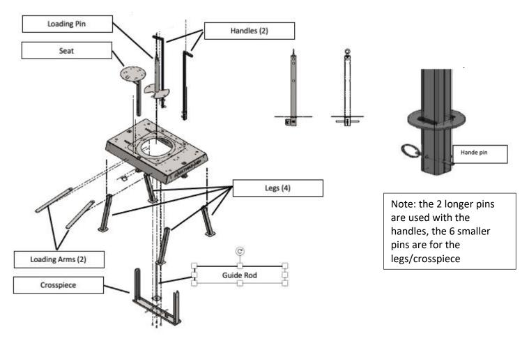
The guide rod is the only part that requires a tool (flat head screwdriver). 4 bolts are used to mount in the crosspiece. The "BLACK" limiting strap attaches onto the guide rod and loading pin hooks to keep the loading pin from coming off the guide rod. The rubber washer slides over the guide rod and sits at the bottom.
